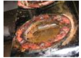
Corrosion to the block from using plain water
